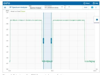
Figure 4. Patent-pending TDD Sync gated sweep feature.
